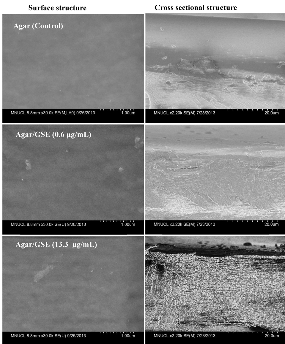
Fig. 4. SEM images of surface and cross section of the agar (control), agar/GSE (0.6 µg/mL) and agar/GSE (13.3 µg/mL) composite films.
